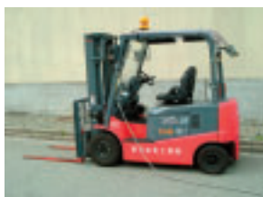
Battery-powered forklift trucks
