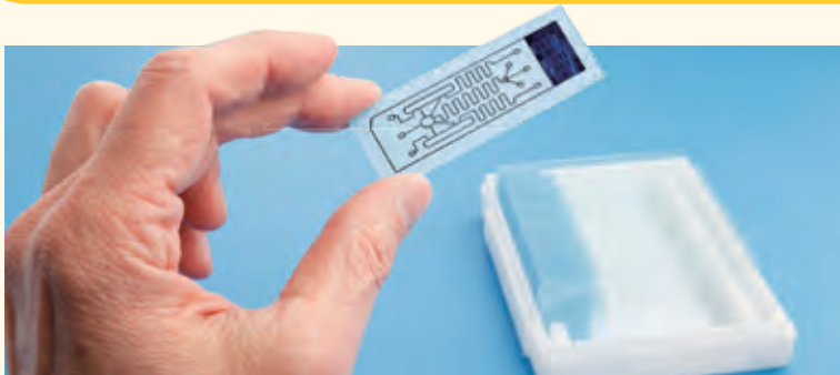
Biochip for a next-generation DNA sequencer *The photo is a sample image.
