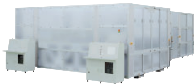
The TR117000 S Spinless® coating machine for 7.5-generation glass substrates
