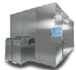
Zero Newton debonding machines TWR series
