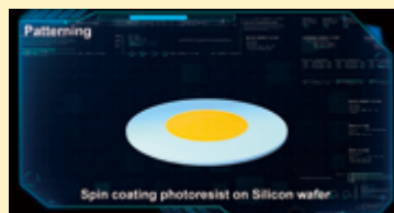
Photoresist patterning process
