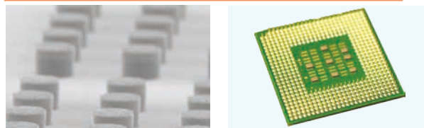
Bumps formed on an IC chip (solder balls) *IC chip photo is an image.
