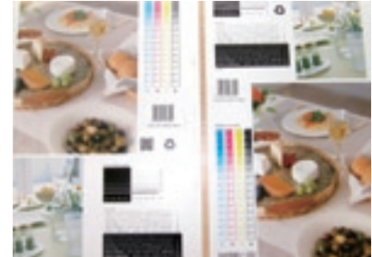
Printing test with reused PS plate Left: Plate used for the first time Right: Printed with reused plate
