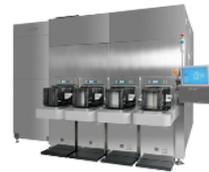
Bonding machine for 3D packaging
